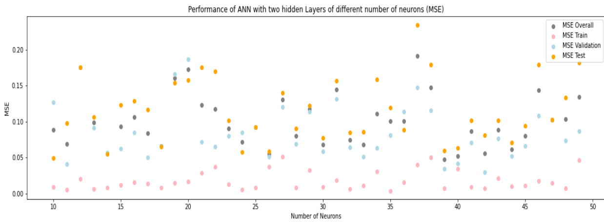
Figure 4.4 ANN performance with respect to varying number of neurons in the second hidden layer. (i) R; (ii) MSE.
